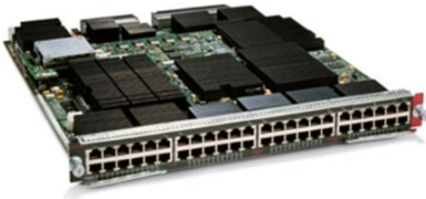
Figure 5. 6800 Series 48-Port 10/100/1000 Interface Copper Module WS-X6848-TX-2T/2TXL
