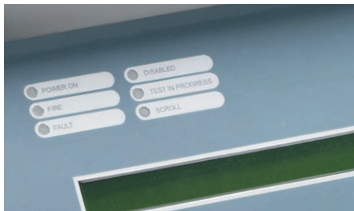
2 x 40 backlit LCD display and 6 supervisory LED's
